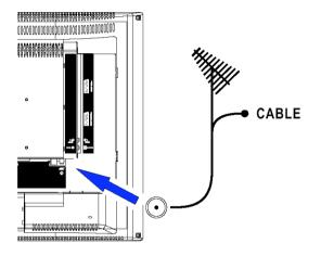
The aerial socket (75 Ohms - VHF / UHF / cable) can be used for connecting an external aerial or other equipment fitted with a modulator (video recorder, satellite receiver, etc.).
